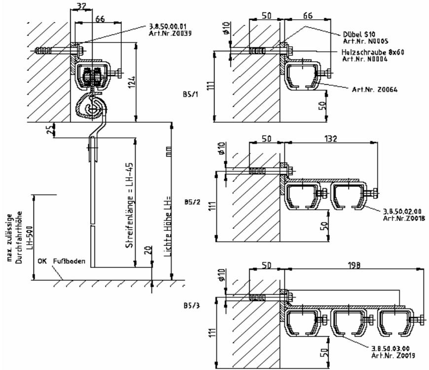
The PVC strips are manufactured with a negative measurement of 20mm. After a few days in heated chambers the strips elongate. After a longer period of time, the PVC strips can have elongated so far, that they stand up on the ground. The strips can be cut simply by using the blade provided.
